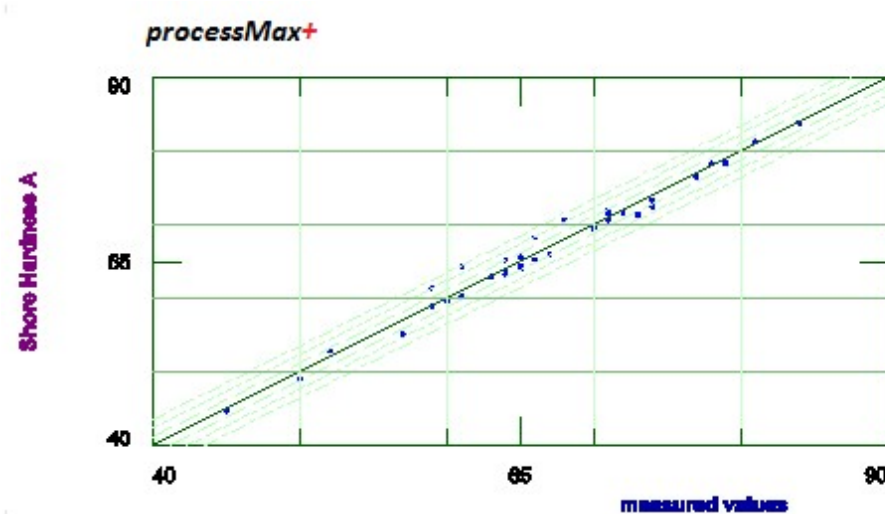
Figure 2. Measured values of hardness against the values predicted by the nonlinear model on the vertical axis
