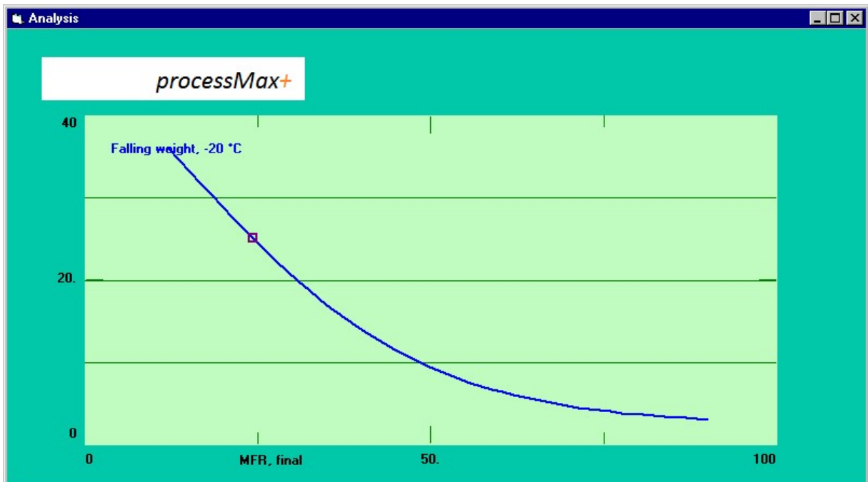
Figure 5. One window in the processMax+ system shows the effect of an input variable on a selected material property.
