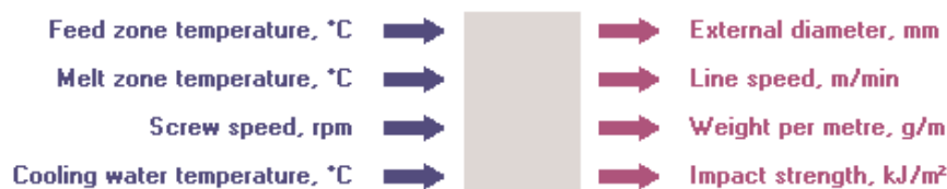
Figure 1. A schematic diagram of models of three properties of extruded pipes and line speed using four process variables as inputs.
